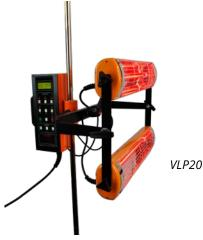
This flexible system allows each cassette to be adjusted and locked into position around the contours of the vehicle body, ensuring maximum area coverage. The drying cycle has all the features of larger systems with flash and bake controls both for temperature and time, automatically switching from flash to bake.
